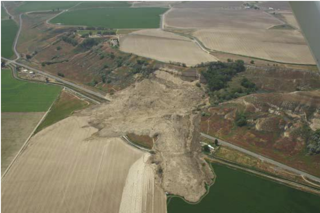
Figure 9.5 Highway 410 Near Town of Nile 2009 5 Landslide Type: Translational
